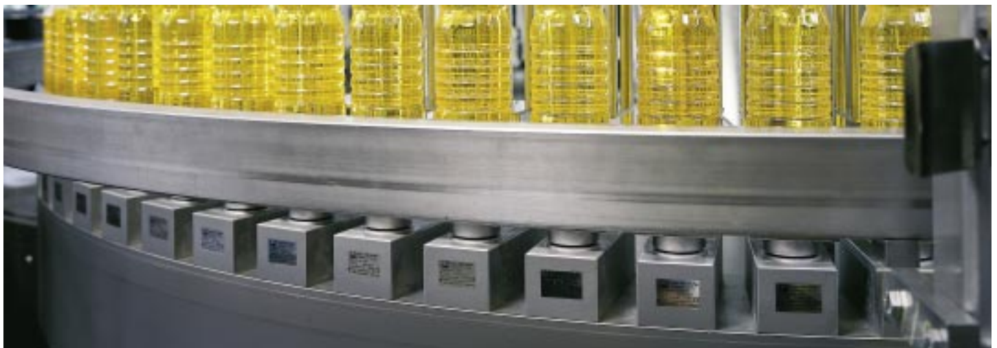
HBM Intelligent Load cells on generic filling machine (not Unilever)
